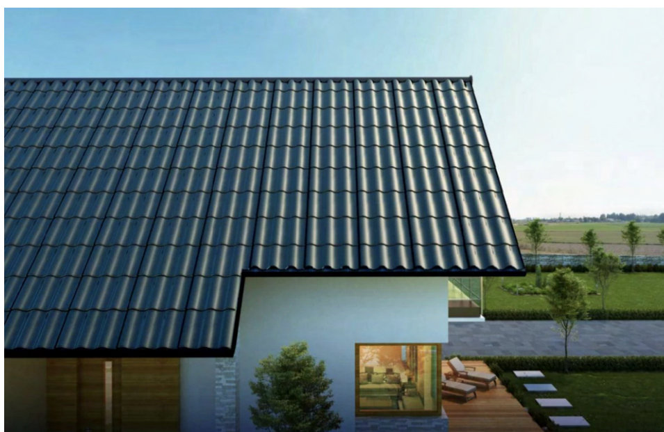
An example of a house roof filled with curved Solar roof tiles.
